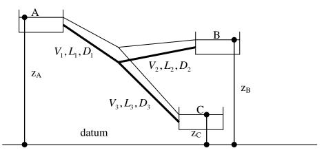
Unknowns:  $V_1, V_2, V_3$ Equations: One continuity and two energy equations
