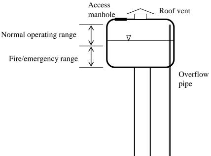
Example: A service reservoir is to be designed for a water-supply system serving 250,000 people with an average demand of 600L/d/capita and a needed fire flow of 37000 L/min. Estimate the required volume of service storage.
