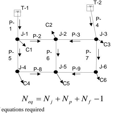
$N_{eq}$ = Number of equations required  $N_j$ = number of junction nodes  $N_l$ = number of loops  $N_f$ = number of Fixed Grade Nodes (e.g. elevated reservoirs)
