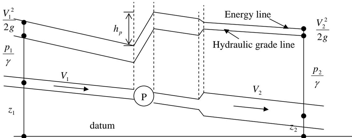
$$z_1 + \frac{p_1}{\gamma} + \frac{V_1^2}{2g} + h_p = z_2 + \frac{p_2}{\gamma} + \frac{V_2^2}{2g} + h_L$$
