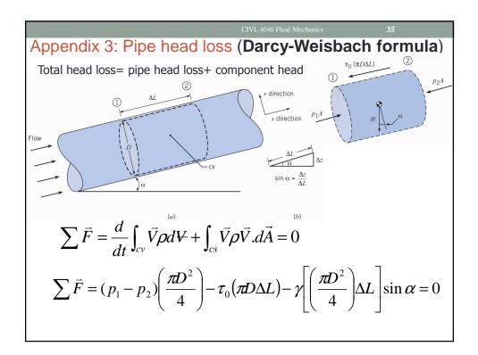
$$(p_1 + \gamma_{z_1}) - (p_2 + \gamma_{z_2}) = \frac{4\Delta L \tau_0}{D} \qquad \left(\sin \alpha = \frac{\Delta z}{\Delta L}\right)$$
