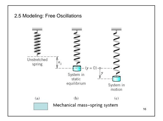
How can we obtain the motion of the body, say, the displacement y(t) as function of time t? Now this motion is determined by **Newton's second law**
